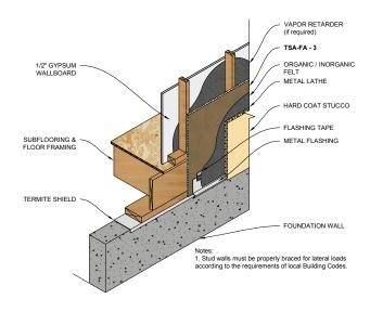
**Re-Siding Construction** - TSA-FA-3 may be used in retrofit construction provided the existing siding is sound and solidly attached. It is secured with galvanized nails of sufficient length to penetrate the old sidings, sheathings below and at least one inch into the existing wall studs. Then, cover the TSA-FA-3 with a suitable new siding of aluminum, vinyl, fiber cement, wood or wood fiber based products.
