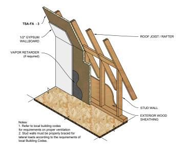
Attics and Crawl Spaces - TSA-FA-3 may be applied to the interior face of stud walls or roof rafters within attics and crawl spaces to provide a layer of continuous insulation (ci). Simply nail the TSA-FA-3 to the framing members and cover with an approved ignition barrier such as 3/8" gypsum wallboard or 1/4" wood structural panel, particle board or hardboard.
