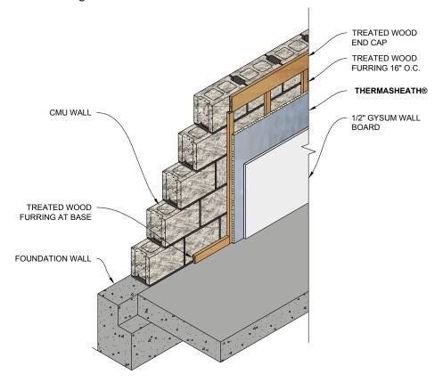
Refer to Thermasheath<sup>®</sup> Product Data Sheet for additional application/installation, compliances, thermal and physical properties, limitations and warnings.
