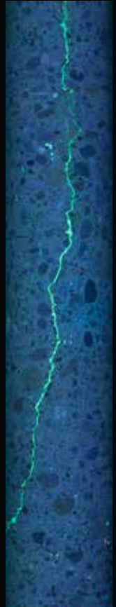
This concrete core sample shows a 24" full depth repair using Roadware Easy Injection Cartridges..
