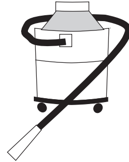
Shop vacuum for cleaning out dust and debris from cracks and spalls
