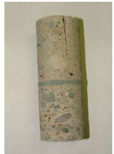
Fig. 3: Cores drilled after the repair is complete are used to verify that the repair was successful
