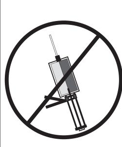
CAUTION: DO NOT POINT MIXER UPWARD AFTER MATERIAL IS FLOWING! This may cause Back-flo and clogging.
