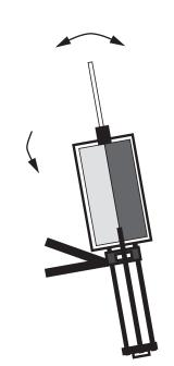
Hold cartridge upward and load into gun. Bleed off any air inside the cartridge by slightly squeezing handle and rocking the cartridge from side to side as needed to force the air bubble out through the mixer.
