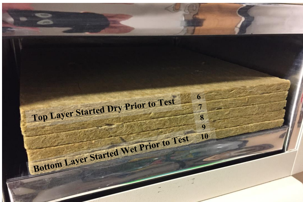
Figure 14: Five samples of ROCKWOOL® stone wool insulation about to be tested in C518 apparatus. Moisture concentrated in the bottom layer at start of test.
