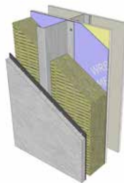
Vertical Z-girt over steel stud wall assembly. Girts are fastened to studs behind at every 16" o.c. resulting in significant thermal bridging through the exterior insulation.
