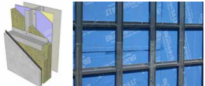
Crossing Z-girt assembly consisting of horizontal and vertical Z-girts attached at crossing points.
