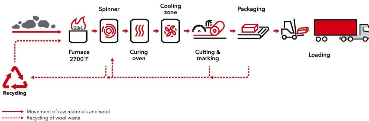
Figure 4: Manufacturing process of ROCKWOOL stone wool insulation
