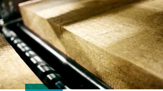
FABROCK<sup>™</sup> DD is a dual-density stone wool board insulation that is designed to be fabricated while maintaining its integrity. A high-density layer and a lower-density layer work together to give the product compressive resistance and excellent sound absorbency.
