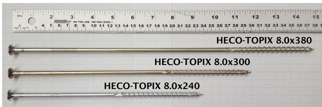
Figure 2.7 HECO-TOPIX 8.0x screws used in this testing
