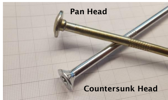
Figure 3.4 Photo comparing countersunk and pan head screws
