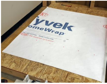
Figure 2.2 Backup wall framing sheathed with OSB and Tyvek HomeWrap stapled to OSB
