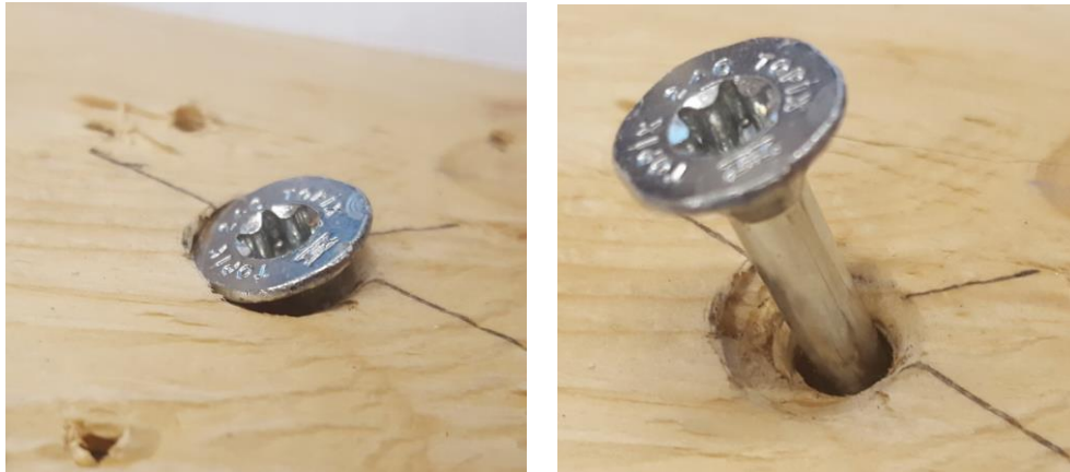
Figure 3.18 Close-up photos of 3/4" plywood strapping at a screw penetration Note the slight bearing damage on the strapping.
