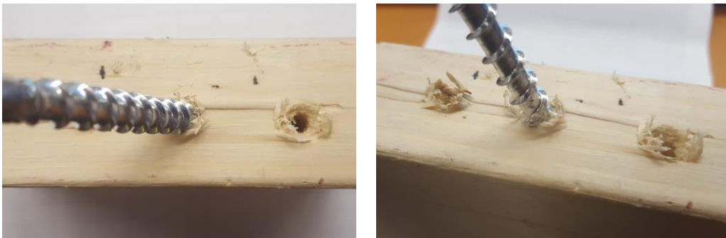
Figure 3.17 Close-up photos of backup wall framing at screw penetrations after screw bending test
