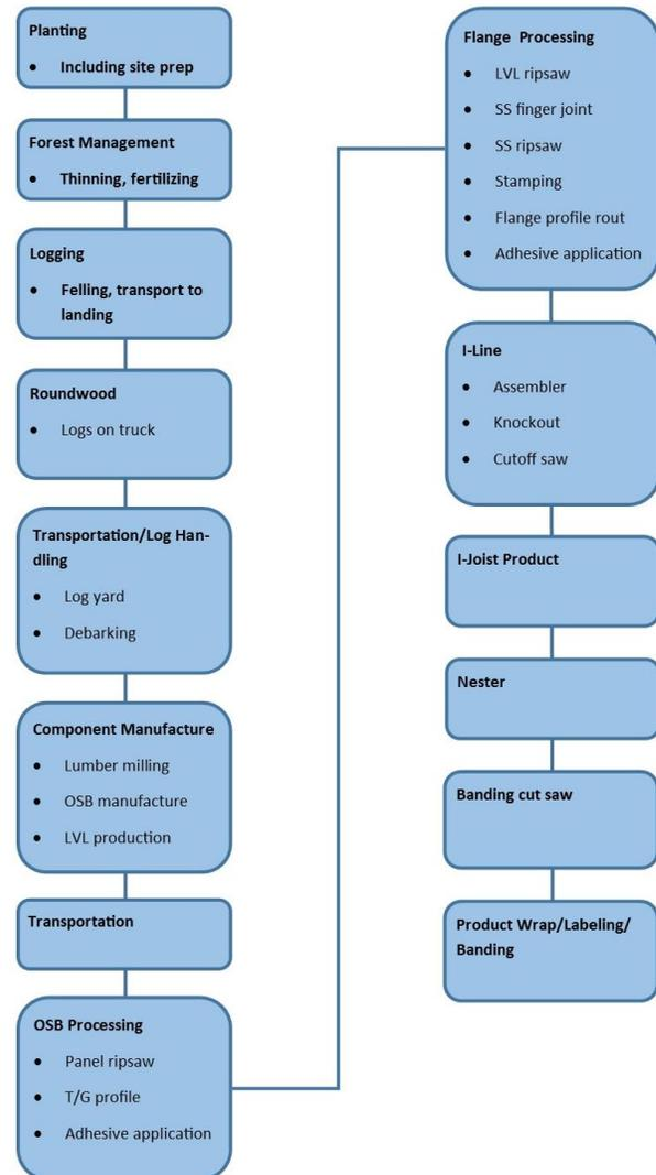
Figure 1: Cradle-to-gate product system for I-joist
