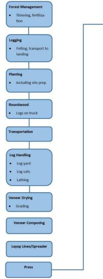
Figure 1: Cradle-to-gate product system for hardwood plywood
