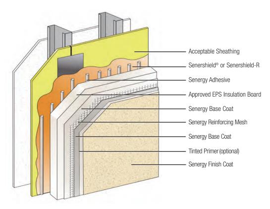
Senerflex Channeled Adhesive Design over metal studs
