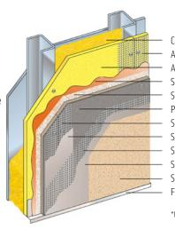
Cavity Insulation\* Approved Joint Reinforcement Acceptable Sheathing\* Senershield-R/-RS/-VB SikaWall Drainage Mat PermaBASE CI™ Insulation Cement Board\* SikaWall Self Adhering Mesh Tape Senergy Base Coat Senergy or SikaWall Reinforcing Mesh Senergy Base Coat Senergy Finish Flashing or Starter Track\*
