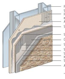
Framing\* SikaWall MaxFlash, SikaWall FlashSeal NP or SikaWall Sheathing Fabric embedded in Senershield-R,-RS, or -VB Acceptable Sheathing\*
