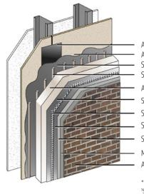
Approved Joint Reinforcement<sup>†</sup> Acceptable Substrate\* Senershield-R/-RS/-VB Senergy Adhesive
