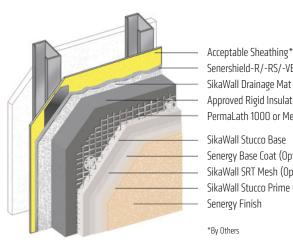
Senershield-R/-RS/-VB SikaWall Drainage Mat Approved Rigid Insulation Boar PermaLath 1000 or Metal Plaster Base
