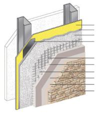
Approved Substrate\* Senershield-R/-RS/-VB SikaWall Drainage Mat DF Approved Joint Reinforcement
