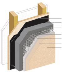
Acceptable Sheathing\* Water-Resistive Barrier\* Approved Rigid Insulation Board\* Permalath 1000 or Metal Plaster Base\* SikaWall Stucco Base SikaWall Stucco Prime (Optional) Senergy Finish
