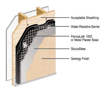
Sentry Stucco Wall System is a Portland cement-based exterior wall system.
