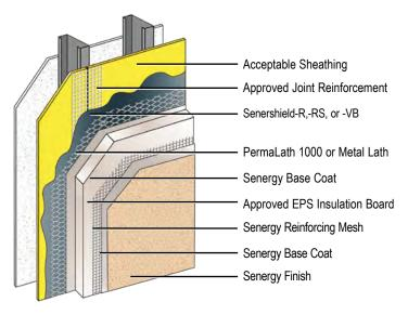
Adhered Mat Design is an EIFS with drainage incorporating an unobstructed drainage plane and an air/water-resistive barrier that provides maximum wind load resistance.
