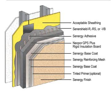
Senergy Platinum CI (Continuous Insulation) is an exterior cladding system featuring Neopor<sup>®</sup> advanced insulation technology.
