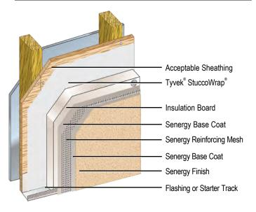
Senturion I is a mechanically attached Class PB EIFS with drainage incorporating Tyvek StuccoWrap water-resistive barrier.
