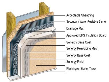
Senturion III is a mechanically attached Class PB EIFS with drainage incorporating a pre-formed drainage mat and a waterresistive barrier to provide an unobstructed drainage plane.
