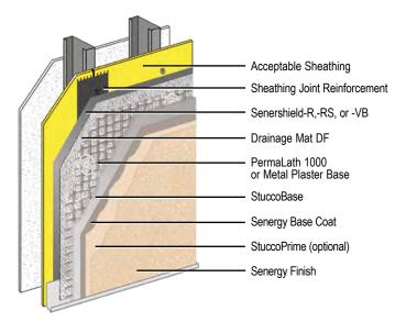
Sentry Stucco Ultra is a highly advanced Portland cementbased exterior wall system. Its features a rainscreen design for maximum water management security, a fluid-applied air/waterresistive barrier, drainage mat, available rustproof fiberglass lath, a base coat and textured finishes.
