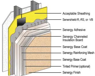
Channeled Insulation Design is an adhesively attached, continuously insulated water-drainage exterior cladding incorporating channeled EPS insulation boards and a secondary air/water-resistive barrier for added water management security.
