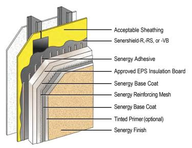
Channeled Adhesive CI Design is an adhesively attached, continuously insulated water-drainage exterior cladding incorporating vertical drainage channels and a secondary air/water-resistive barrier.
