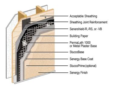
Sentry Stucco Plus is a highly advanced Portland cement-based exterior wall system. It features a fluid-applied air/water-resistive barrier, available rustproof fiberglass lath, a base coat and textured finishes.
