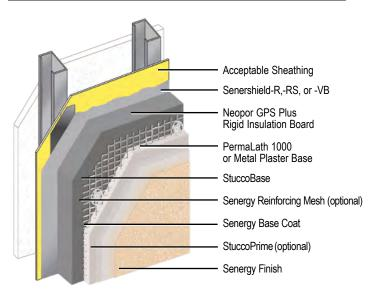
Senergy Platinum CI Stucco Plus is a premium continuously insulated cement plaster/stucco featuring Neopor GPS Plus Rigid Insulation Board and a fluid-applied air/water-resistive barrier.
