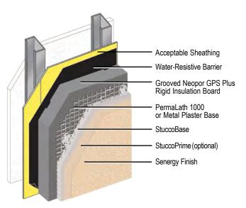
Senergy Platinum CI Stucco is a continuously insulated cement plaster/stucco system featuring Neopor GPS Plus Rigid Insulation Board.
