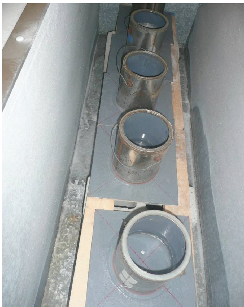
ASTM D1970 test apparatus. This test measures the ability of a barrier material to self-seal around two nails in a manner sufficient to prevent a column of water from seeping through the penetration.
