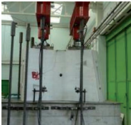
Figure 18 : Point load test set-up
