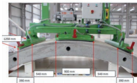
Figure 21 : Vacuum lifting system
