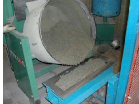
Figure 36: Filling the mould of an EN14651 beam
