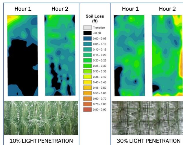
Figure 1 - Light Penetration Comparison
