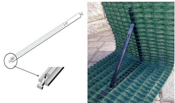
Figure 1 - Fiber-composite bars are threaded through the fabric and snapped together to form an internal brace
