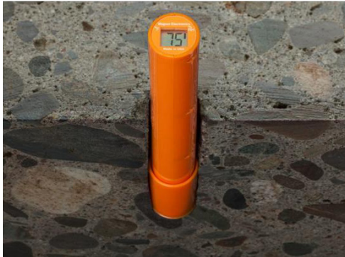
Relative Humidity (RH) ASTM F2170
