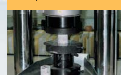
Compressive strength of core sample Compression press 5
