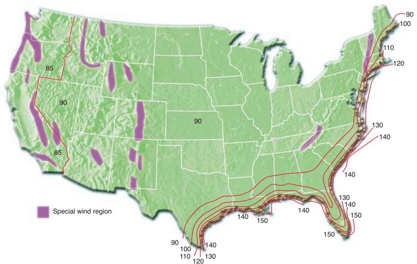
Typical Wind Map — used by roofing designers to identify wind velocity zones.
