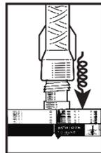
**3. Attach** — Attach proper Simpson Strong-Tie® nozzle and extension to cartridge. Do not modify nozzle.
