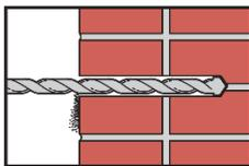
**1. Drill** — Drill 1-inch-diameter hole to specified depth with a carbide-tipped drill bit, using rotation only mode. For Configuration A, drill 8 inches deep. For Configuration B, drill to within 1 inch of the opposite side of wall (minimum 13 inches deep).
