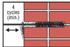
**3. Brush** — Clean with a 1-inch-diameter nylon brush for a minimum of four cycles. Brush **MUST** reach the bottom of the hole. Brush should provide resistance to insertion. If no resistance is felt, the brush is worn and must be replaced.
