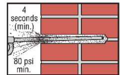
**4. Blow** — Remove dust from hole with oil-free compressed air for a minimum of 4 seconds. Compressed air nozzle **MUST** reach the bottom of the hole.
