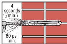
**2. Blow** — Remove dust from hole with oil-free compressed air for a minimum of 4 seconds. Compressed air nozzle **MUST** reach the bottom of the hole.
