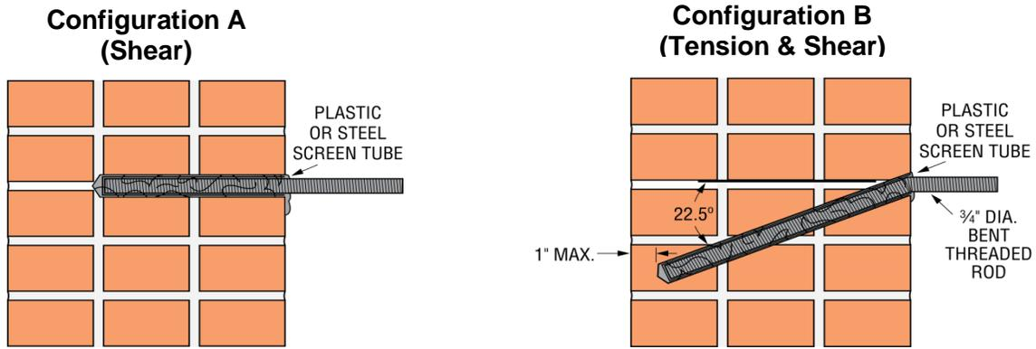
**FIGURE 1—ANCHOR INSTALLATIONS FOR UNREINFORCED BRICK MASONRY**
