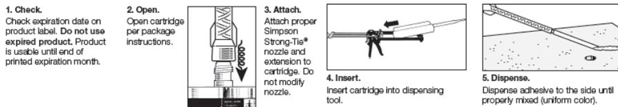
Note: Review MSDS prior to use. Refer to Tables A, B and C for proper nozzle and dispensing tool part number. Refer to Tables F and G for proper adhesive storage temperatures, permitted concrete temperature range and adhesive gel times.
