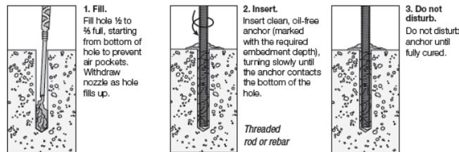
Note: Refer to Table F for proper gel times and cure times and Table D and E for maximum tightening torque. Nozzle extensions may be needed for deep holes.
