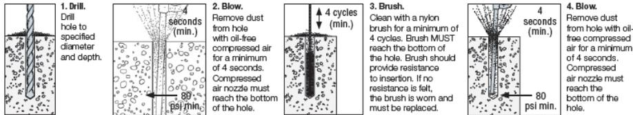
Note: Refer to Tables A, B, and C for proper drill bit size and brush part number.
