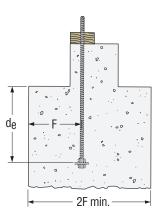
Design loads are calculated using a full shear cone. Coverage on each side of the bolt shall be a minimum of F or reductions must be taken.
