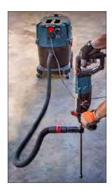
Approved for installation with multiple vacuum drill bit systems.\*
