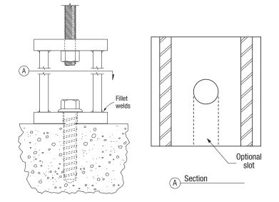
**Note:** Torque-testing of anchors is not considered to be a suitable method of verifying anchor tension capacity since the torque-to-tension relationship of concrete anchors varies depending on installation and base material conditions.
