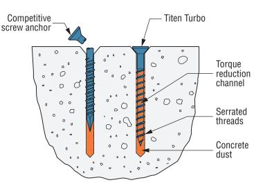
Patented Torque Reduction Channel Displaces Dust for Trouble-Free Installation SIMPSON
