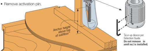
\*Anchor Rod extension above top of subfloor considers 2x nominal sole plate thickness. Increase as required for not or 4x sill plates, bottom plates, and for holdowns raised off of sole plate.
