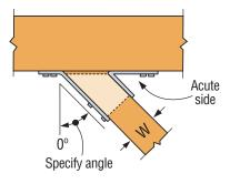
Top View HHUS Hanger Skewed Right (joist must be bevel cut)
