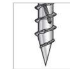
Sharp Point with Nib Application: Wood, composite
