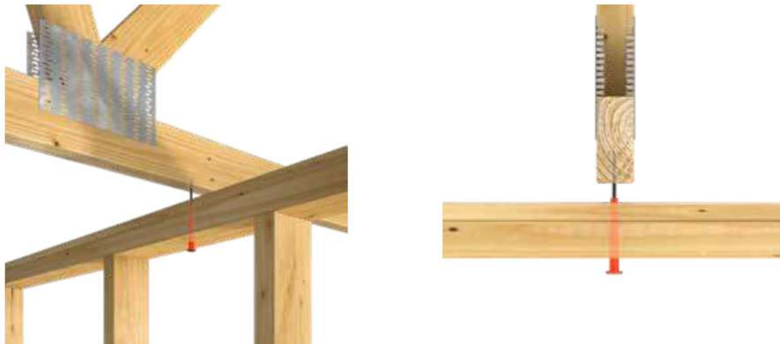
Typical Installation of SDPW DEFLECTOR Screws
