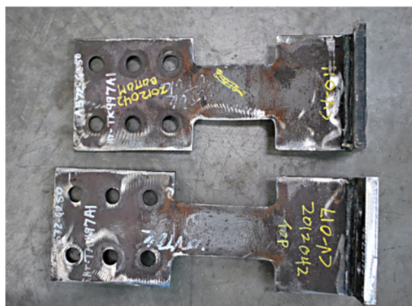
Sample Yield-Link Compression and Elongation from Testing
