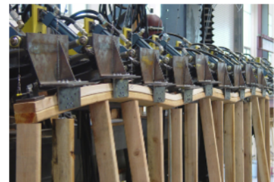
Top-Plate Bending Due to Uplift
