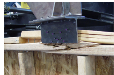
Failure at Top-Plate Splice
