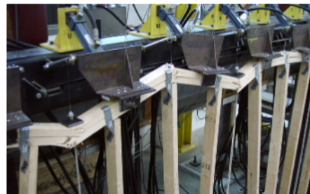
Ultimate Failure of Top Plate in Pure Bending Due to Rotation Restraint
