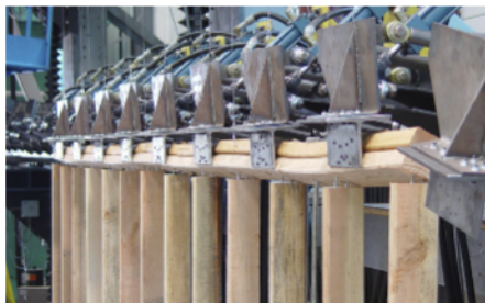
Top-Plate Rotation Failure Due to Uplift
