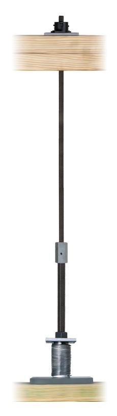
To ensure structural stability, a continuous rod tiedown system can be used in wood-framed structures to resist shearwall overturning and roof uplift. Simpson Strong-Tie Strong-Rod systems provide both an anchor tiedown system (ATS) for shearwall overturning restraint and an uplift restraint system (URS) for roofs.
