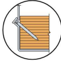
Correct Nailing Approx. 45° Angle
