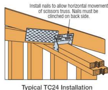
Typical TC24 Installation
