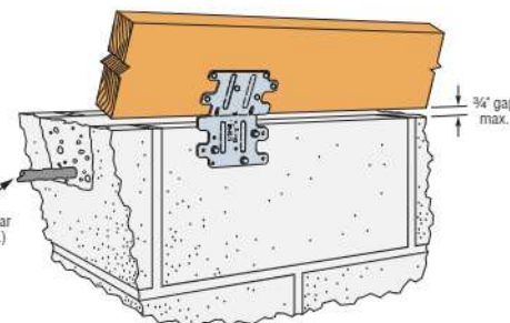
3 Typical RBC Installation to GFCMU Block (RBCP similar)
