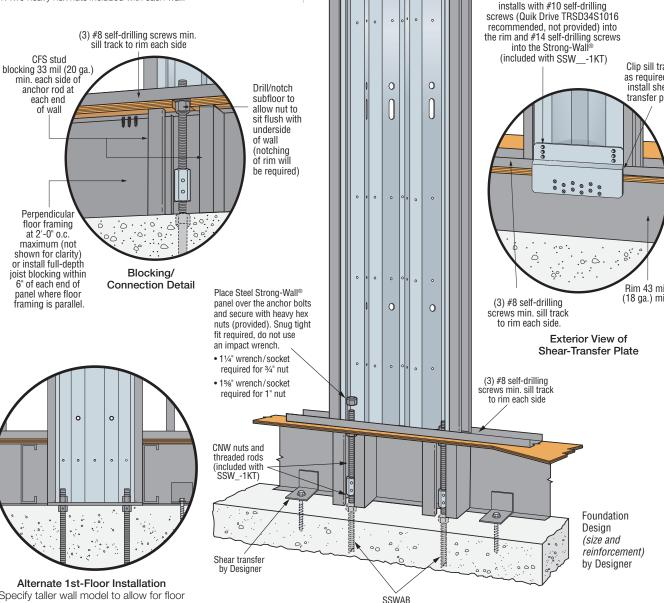
Specify taller wall model to allow for floor framing and use load values for installation on concrete; see pp. 286-287.
