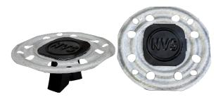
The Siplast NVS Fastener is formed from specially coated galvanized steel. The split-wedge leg spreads upon installation into lightweight insulating concrete to provide withdrawal resistance. NVS Fasteners are assembled to incorporate a corrosion resistant Galvalume® coated stress distribution plate.
