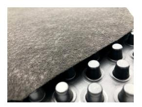
Paradrain W Drainage Mat is a dual-component prefabricated sheet drain and protection board consisting of a formed polypropylene core covered on one side with a woven polypropylene filter fabric. The fabric allows water to pass into the drain core while restricting the movement of backfill materials or debris that could potentially block the core. The core allows water flow to designed outlets.
