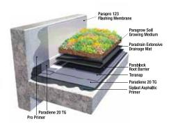
Teranap Intensive Green Systems are used to waterproof elaborately designed roofscapes that are intended for pedestrian access. In an intensive system, soil depth starts at 8 inches. Therefore, a more diverse plant selection, including trees and shrubs, is possible. The wet weight of intensive systems typically starts at 50 lb/sq ft, so they must be engineered to conform to structural load requirements. Intensive green systems require regular maintenance and watering.
