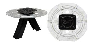
The Zono-Tite Fastener is formed from specially coated galvanized steel. The split wedge leg spreads upon installation into lightweight insulating concrete to provide withdrawal resistance. Zono-Tite Fasteners are assembled to incorporate a corrosion resistant Galvalume-coated stress distribution plate.
