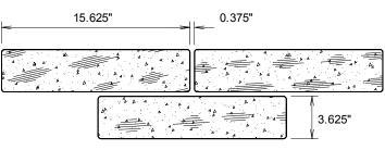
**ATTACHMENT TO FORMWORK** – Liners are attached to the form using TEK screws through the face of the liner spaced 12" C-C. Optional form mounting T-nuts embedded through the plywood backing is available for Elastospec panels.
