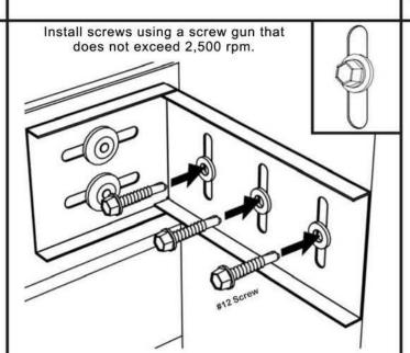
Fasteners should be installed through each step bushing.
