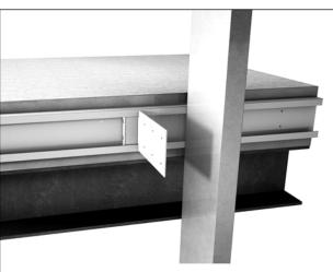
Ensure stiffener is in place prior to installation into track.
