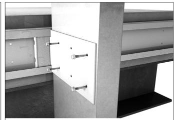
Attach stud to clip with specified fasteners through guide holes.
