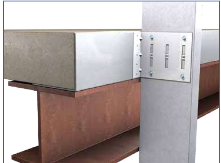
MasterClip® VLB used as a Rigid Connection
