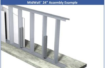
MidWall 24" is generally used in interior half walls of less than 48" in height. Attach MidWall 24" to a 54mil stud with #12 screws through all pre-drilled guide holes. Other studs in the walls are typical infill studs. Maximum spacing between MidWall connectors is 36" o.c. (see table on following page). Contact TSN Technical Services at (888) 474-4876 for design recommendations.
