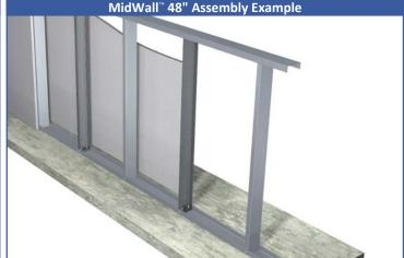
MidWall 48" is used in interior half walls equal to or more than 48" in height. Use one MidWall 48" as a substitute for a stud at the specified spacing, or attach to a 54mil stud with #12 screws through all pre-drilled guide holes. Maximum spacing between MidWall connectors is 36" o.c.
