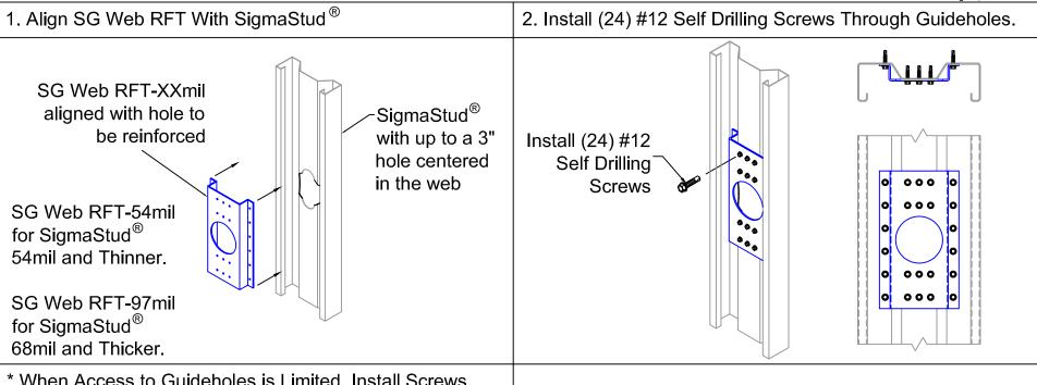
\* When Access to Guideholes is Limited, Install Screws Between Guideholes From Opposite Side.
