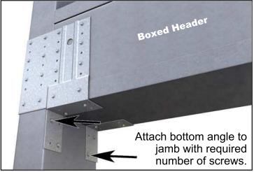
Consider using TSN's JamStud® in place of all window or door jamb studs for added quality. For Installation, Technical or Submittal questions, contact The Steel Network at **(888) 474-4876** or email us at **support@steelnetwork.com.**
