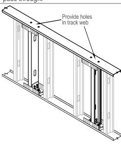
⑤ Install anchors or through rods into the top base plates. If another floor is to be added, and through rods are used, they will extend through the floor and into the lower StiffWall® boot assembly of the next
