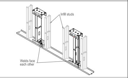
④ Install top track. Track web holes must be provided at boot assembly locations for upper floor anchors to pass through.
