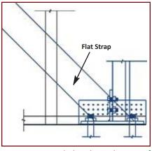
It is recommended to limit the use of 10" flat strap to shear wall panels that have aspect ratio > 0.72:1 (36 degrees)
